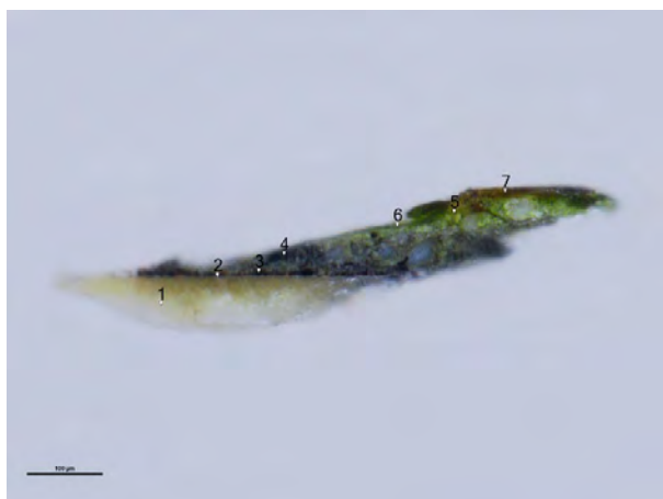
A1.3 Lucas Cranach the Elder, Adam and Eve , National Museum in Warsaw, stratigraphy of sample C7: 1) white ground layer, 2) white imprimatura, 3) underlayer for dead colouring, black, 4) underpainting layer – dead colouring, dark grey, 5) modelling layer, green, 6) discontinuous green layer, 7) discontinuous light brown layer photo Justyna Kwiatkowska
