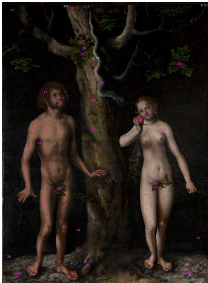
fig. 8 Lucas Cranach the Elder, Adam and Eve , National Museum in Warsaw, map of XRF measurement points (nos 1–36) and micro-sample locations for microchemical (nos C1, C3, C5, C6) and stratigraphic analyses (nos C7, C8, C11) photo Justyna Kwiatkowska
