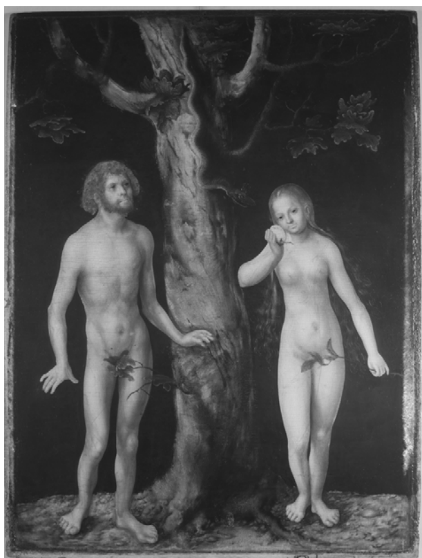
fig. 5 Lucas Cranach the Elder, Adam and Eve , National Museum in Warsaw, X-radiograph of the painting revealing the horizontal butt-joints between individual wooden panels of the support and the modelling technique used for the figures of Adam and Eve, with highlights made by using a higher concentration of lead-based pigments; the small white spots, primarily in the lower part of the painting, indicate traces of xylophagous insects photo Łukasz Kownacki
